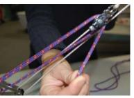
Continue to feed the Dyneema control line back through the bottom block from the starboard side top block in the body of the base unit.
