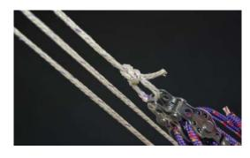
7 Tie the Harken double block to the tail using half hitches or a bowline.
