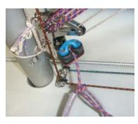
14 Feed the control line through the plastic tube supplied and tie a bowline to form a handle, which is also a stop knot that you can set up to your desired maximum ease setting. Make sure the knot on the block and becket is just short of the top block.
