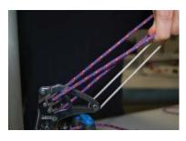
Feed it through the double block from the bottom of the block and through the non-becket side. Make sure the becket is on the port side.
