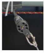
2 Tie the length of **Vectran V12** (1.45 m) in a bowline loop through the top block.
