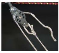
Take the V12 back up to the top block and feed it through from the bottom.
